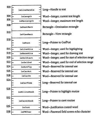
**Figure 34-1** LineEdit edit record (new layout)
