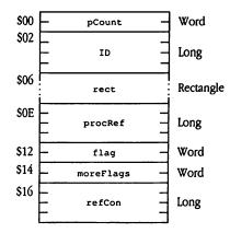
• Figure E-5 Control template standard header
