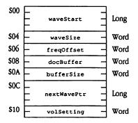
waveStart The starting address of the wave to be played, not in Digital Oscillator Chip (DOC) RAM but in Apple IIGS system RAM. The Sound Tool Set loads the waveform data into DOC RAM as it is played.
