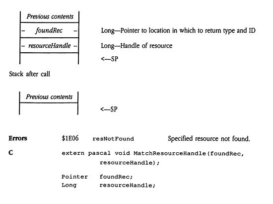
foundRec Must point to a location in memory that can accept 6 bytes of data: the type and ID of the resource in question. On successful return from MatchResourceHandle, that location will contain the following data:
