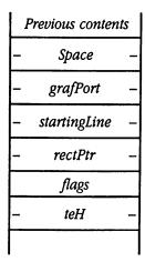
Long—Space for result Long—Pointer to destination GrafPort Long—Starting line number for print operation (0 relative) Long—Pointer to the destination rectangle in GrafPort Word—Control flags for the print operation Long—Handle of TERecord in memory; NIL for active record <—SP
