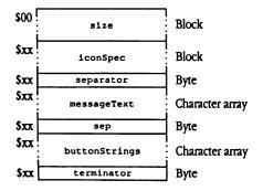
A variable-length block that specifies the size of the alert window to be displayed. Valid ASCII values for the first byte lie in the range from 0 through 9 (\$30 through \$39) and have the following meanings:
