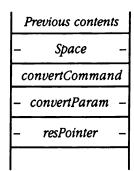
Long—Space for result Word—Command to be performed (will be 0: ReadResource) Long—Pointer to GS/OS read file parameter block Long—Pointer to resource reference record <—SP
