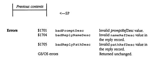
• Note: The GS/OS bufferTooSmall error can occur if the output strings you supply in the reply record are too small to receive the resulting filename string. In this case, the buffer will contain as many name characters as would fit, and the length word will contain the name length the Standard File Operations Tool Set tried to return.
