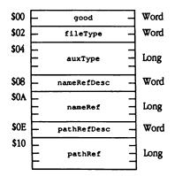
**Figure 48-1** New-style reply record
